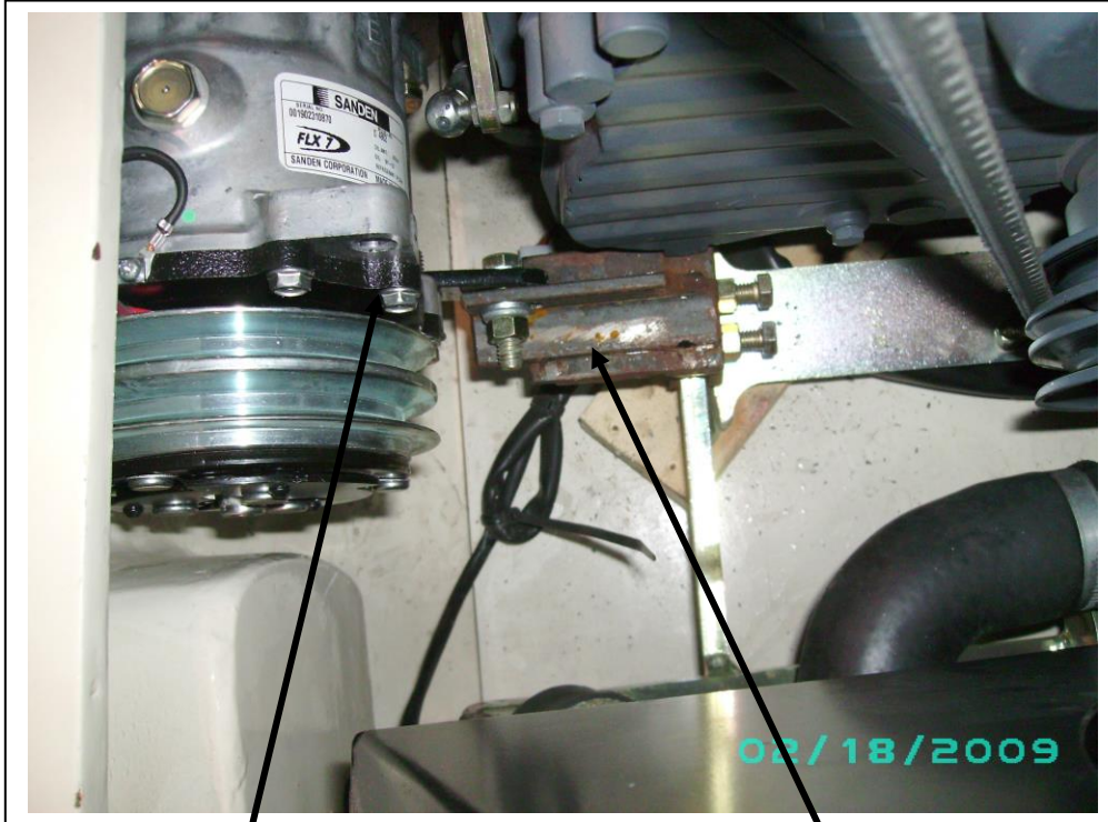
Front bracket mounts to this ear. (Not installed yet in this picture)
