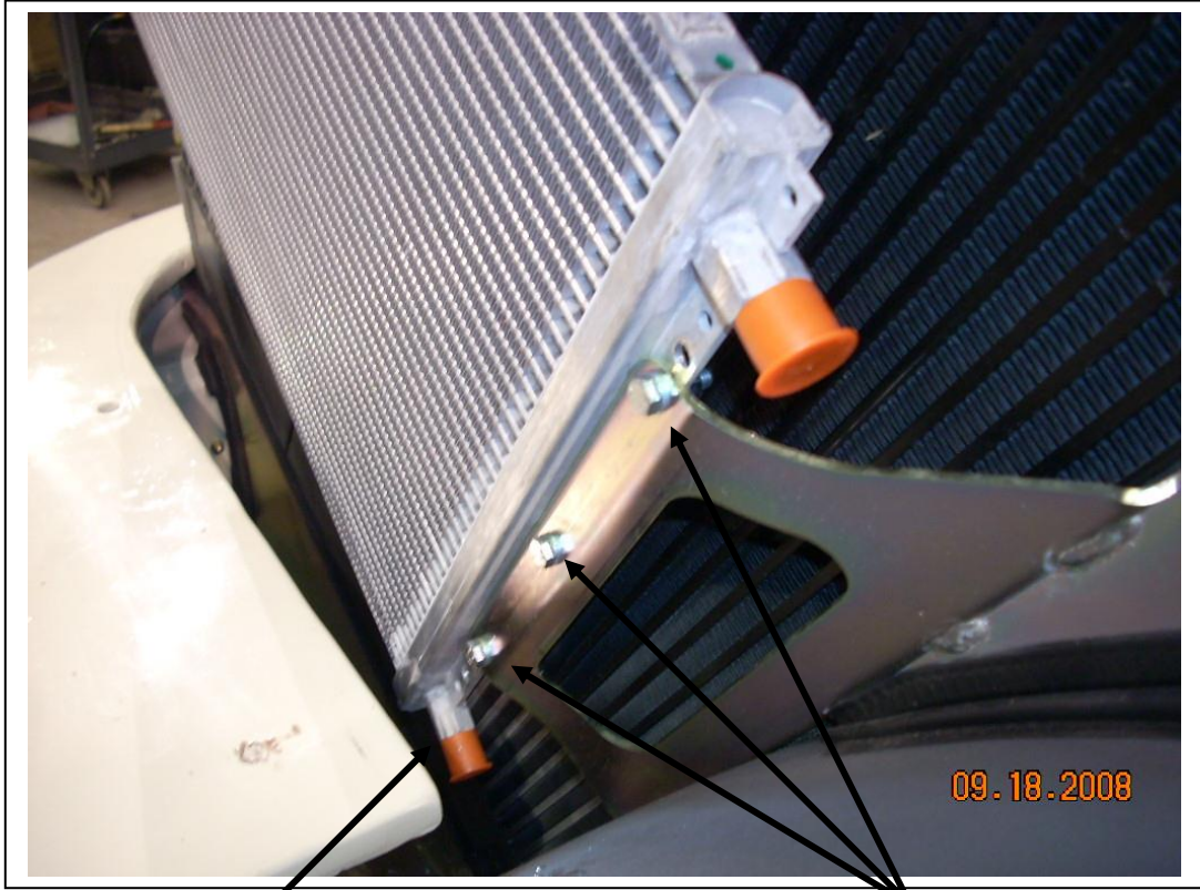
Fitting side of condenser bolts to existing bracket in 3 places.
